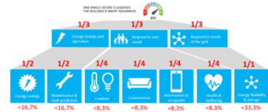
Figure 13 – Aggregation of impact scores to three key functionalities or to a single score
